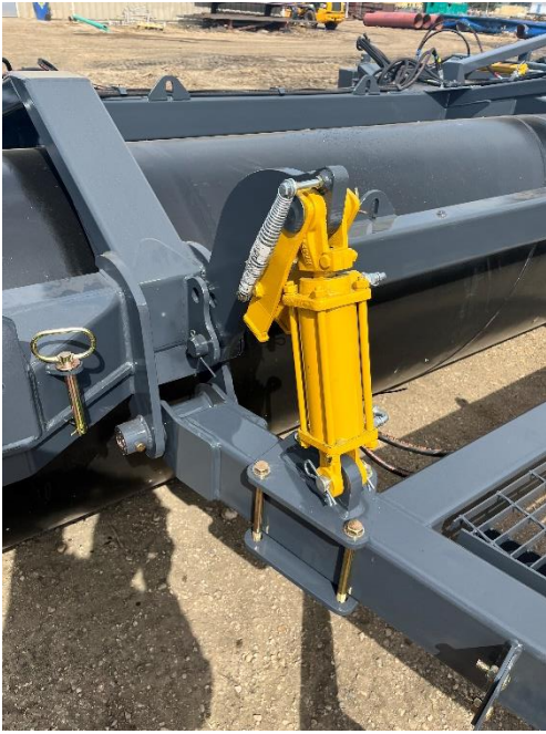
FIGURE 2 CYLINDER LOCKS FOR FLOATING HITCH
