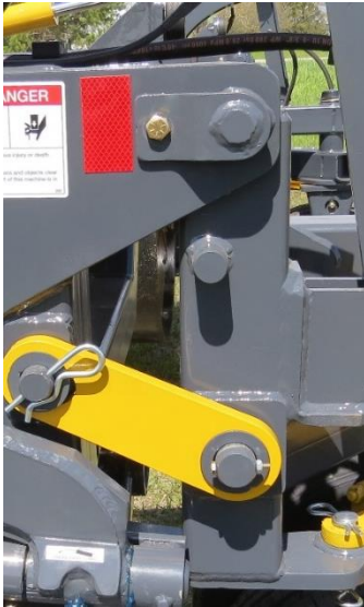
FIGURE 9 DIAGONAL ARM LOCKED
