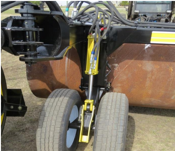
FIGURE 5 CENTER WHEELS UNLOCKED
