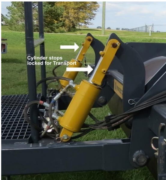
FIGURE 7 TRANSPORT LOCKS FOR HITCH
