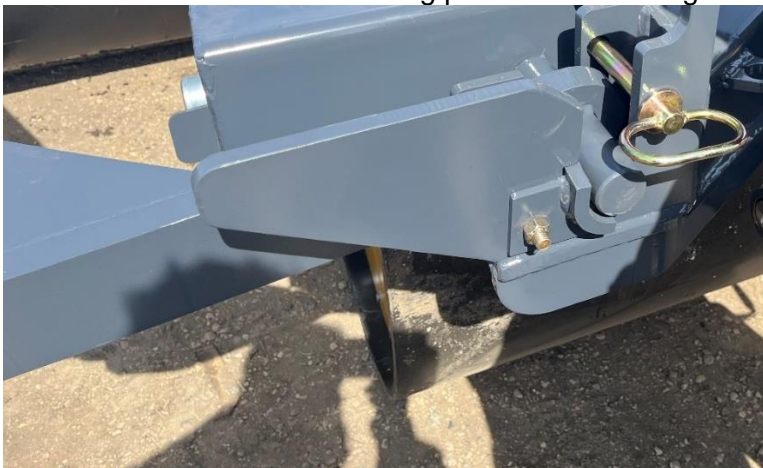
FIGURE 6 PIN FOR DIAGONAL PULL ARM IN LOCKED POSITION
