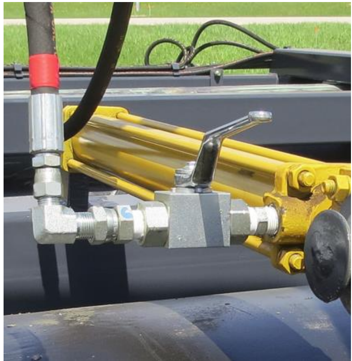
FIGURE 3 FLOATING HITCH PIN REMOVED & HYD VALVE FOR DIAG ARM
