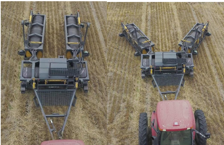
FIGURE 1 WINGS TRAILING DIRECTLY BEHIND & STARTING TO UNFOLD
