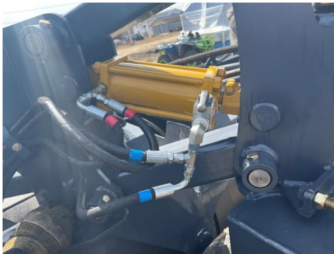
FIGURE 4 REAR TRANSPORT LOCK & CENTER HYD VALVE
