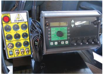
Optional Microtrak autorate controller provides accurate product application. All functions are remotely controlled from the cab by electric solenoids.
