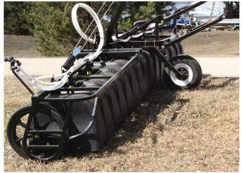
Roadside sprayers feature breakaway booms. The gauge wheels are located at the center and outer edge to ensure booms follow varying terrain.
