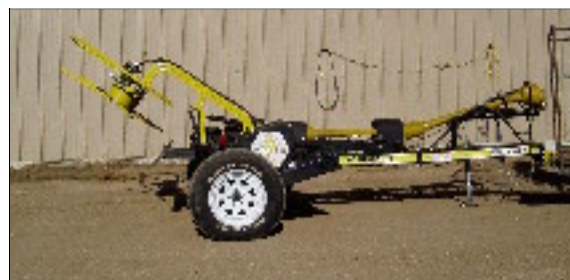
Spinner locked up no spreading
