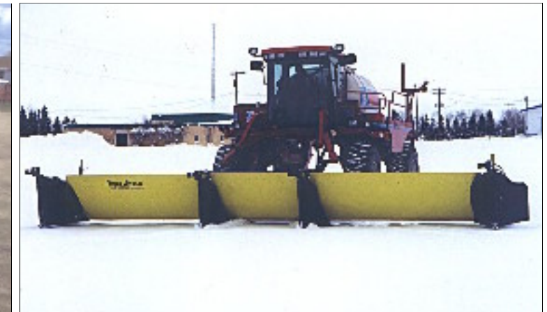
Miller Nitro 275 carrying a Yield Shield on a custom adapter kit.
