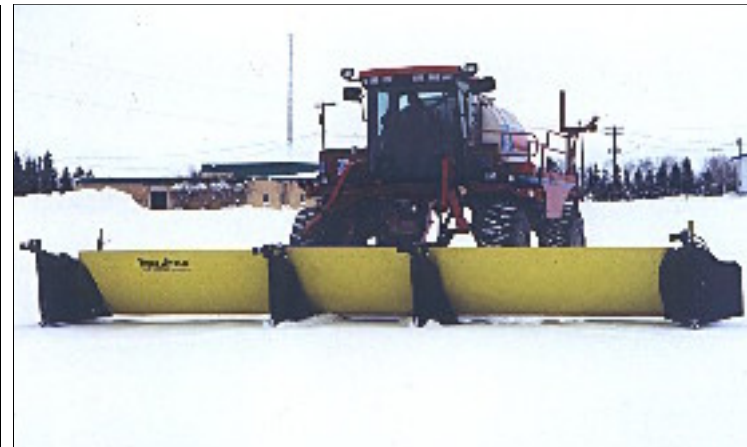
Miller Nitro 275 carrying a Yield Shield on a custom adapter kit.
